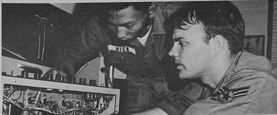
AN OVER-THE-SHOULDER LOOK is one way VNAF technicians learn how to maintain weather equipment. Sgt. Roger D. Friegia, Det. 34, shows VNAF Sergeant Hien where to make an adjustment in a cloud height detecting indicator.
