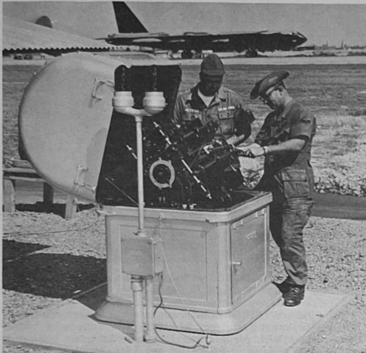
MAKING MINOR ADJUSTMENTS to the projector of the Rotating Beam Ceilometer (cloud measurer) at U Tapao AB, Thailand, are Sergeants Raymond J. Metzger (left) and Robert W. Stalker, both members of Detachment 30, 10th Weather Squadron. Landing in the background is a war-painted B-52 Stratofortress.
