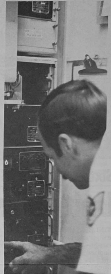
READINGS are being taken from the oblique incidence ionosonde by TSgt. Finley H. Dula during his "watch" at the La Posta, CA, observatory. The oblique incidence ionosonde is a swept frequency receiver which monitors high frequency signals received from Hawaii. (U.S. Air Force photo by TSgt. F. H. Dula)
