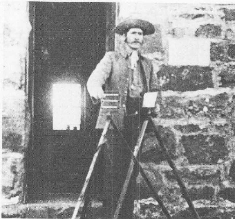
An U.S. Army Signal Corps soldier, at Pikes Peak weather station, transmits latest weather data by heliograph (circa 1880s).
