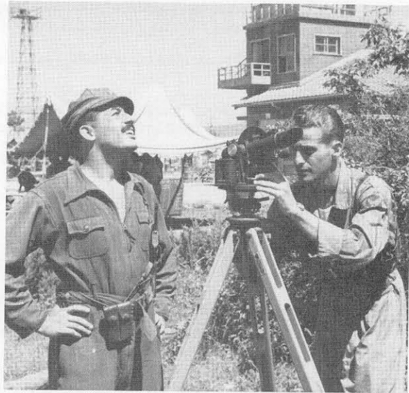
AWS' first Korean War casualty, 1 Lt Grisham, watches Pibal at forward base in Korea in late June 1950 while 20WS' 1 Lt John T. Gordon operates theodolite.
