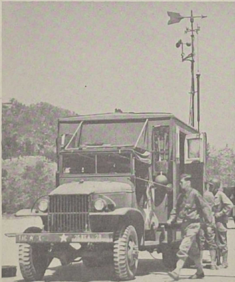
SCM 1 T4 in this picture is the improved mobile station built into a K 53 van. This model is preferred to the T3 because it is far more compact and it operates as a unit.
